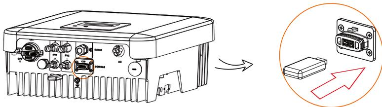
3) Then insert U-disk into the DONGLE port on the bottom of the inverter. Then turn on DC switch or connect the PV connector, the LCD will show the main pictures as below.
