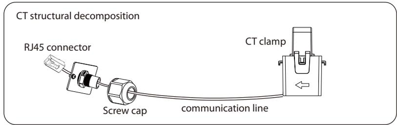
1. Insert the RJ45 connector of CT into the RS485 port on the inverter, and screw down the screw cap tightly.
