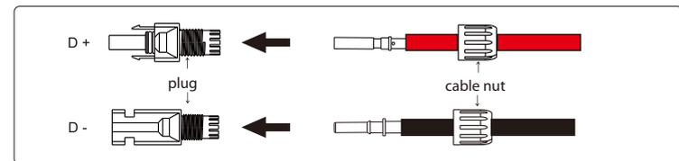
f) Insert the wire into plug forcibly, when a "click" is heard or felt the pin contact assembly is seated correctly. Then tighten the cable nut.
